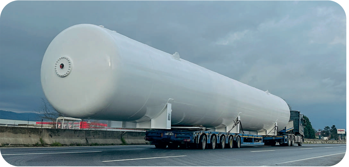
250m 3 Stok Tankı / Storage Tank
