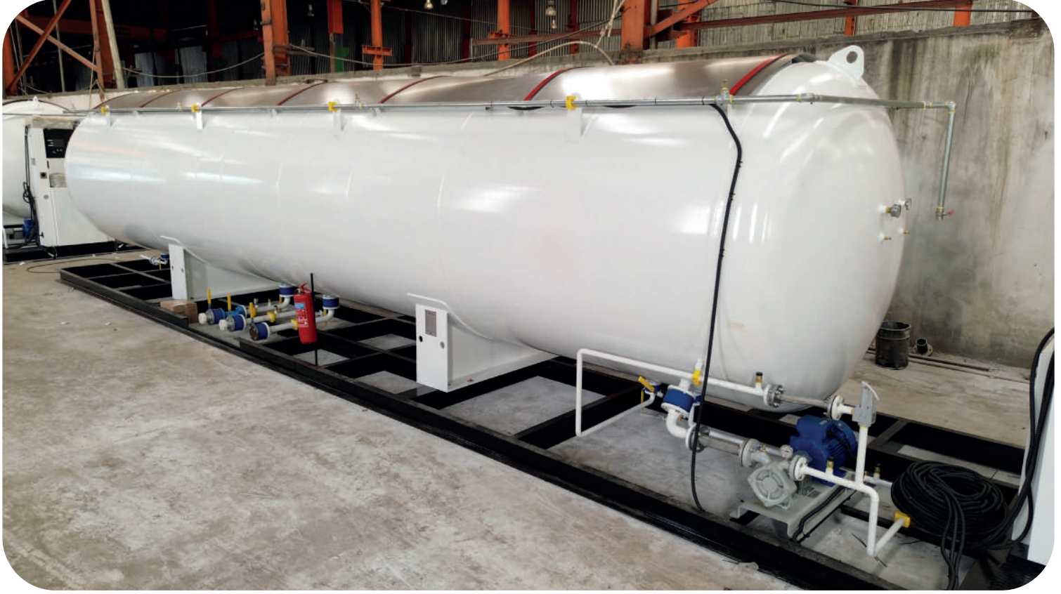
30m 3 LPG Skid Sistem / LPG Skid System
