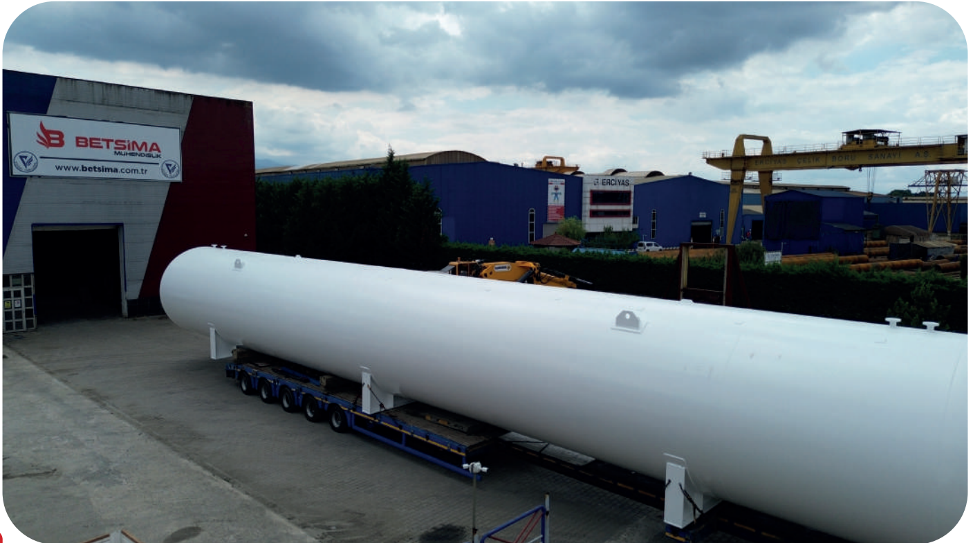
250m 3 Stok Tankı / Storage Tank
