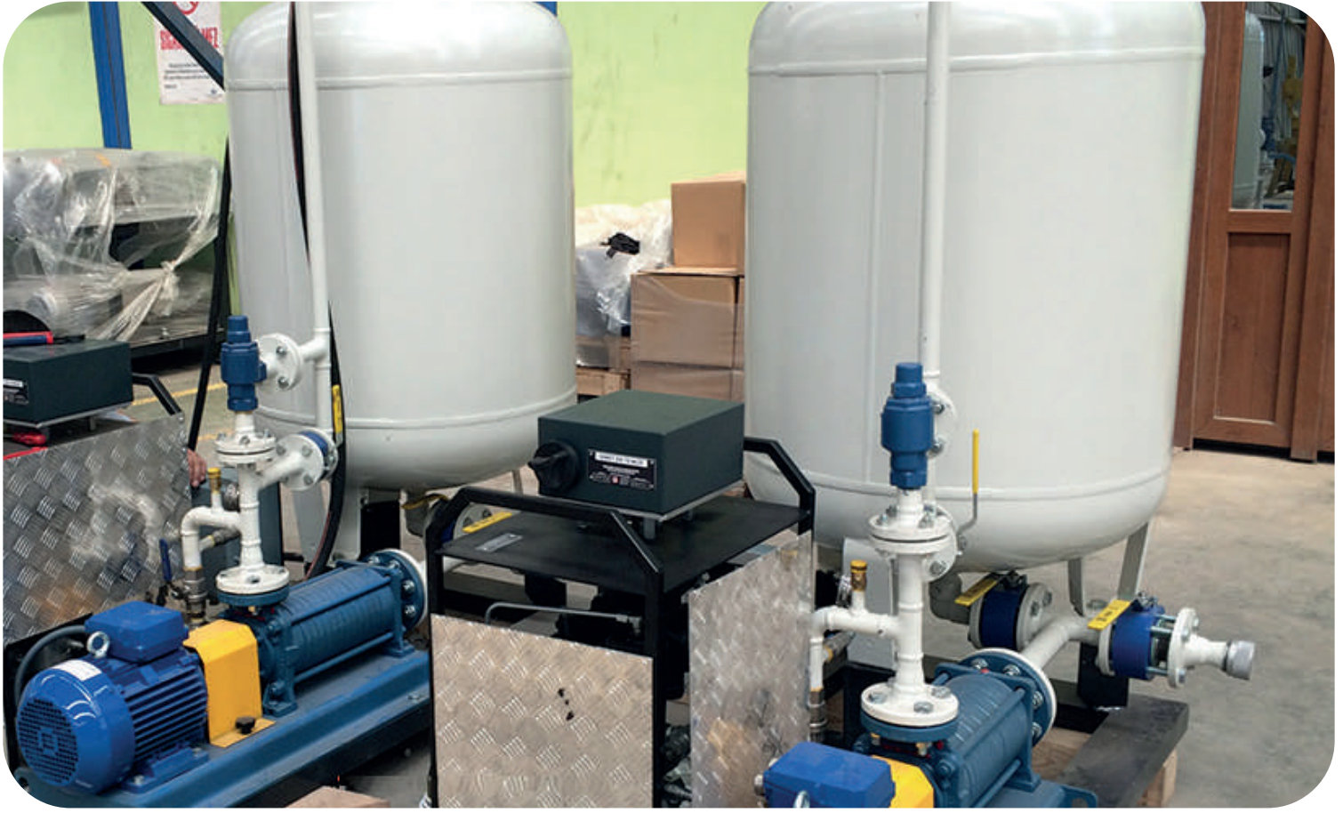
LPG Skid Sistem / LPG Skid System
