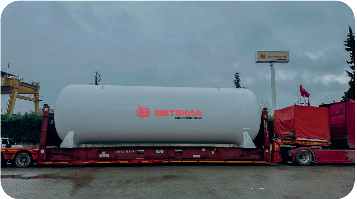
100m 3 Stok Tankı / Storage Tank
