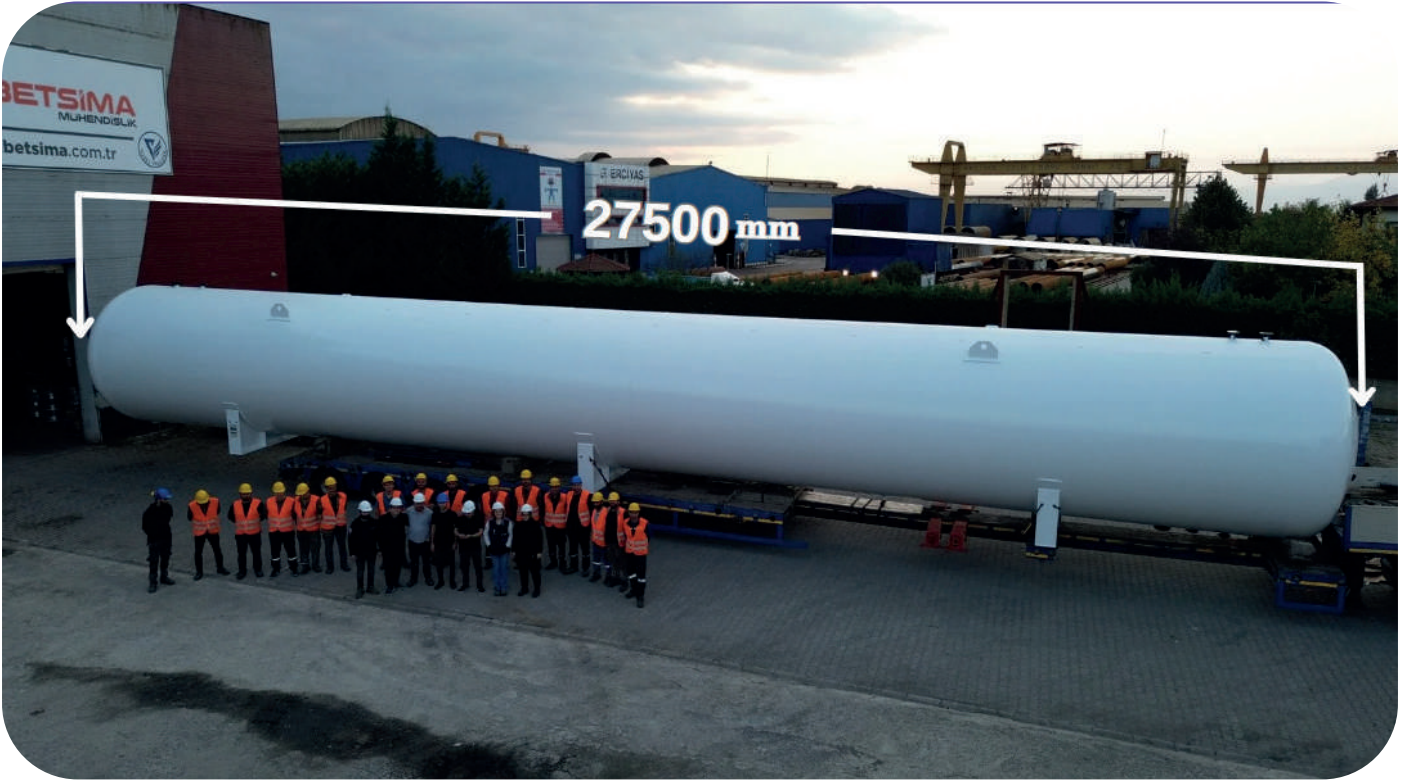
250m 3 Stok Tankı / Storage Tank
